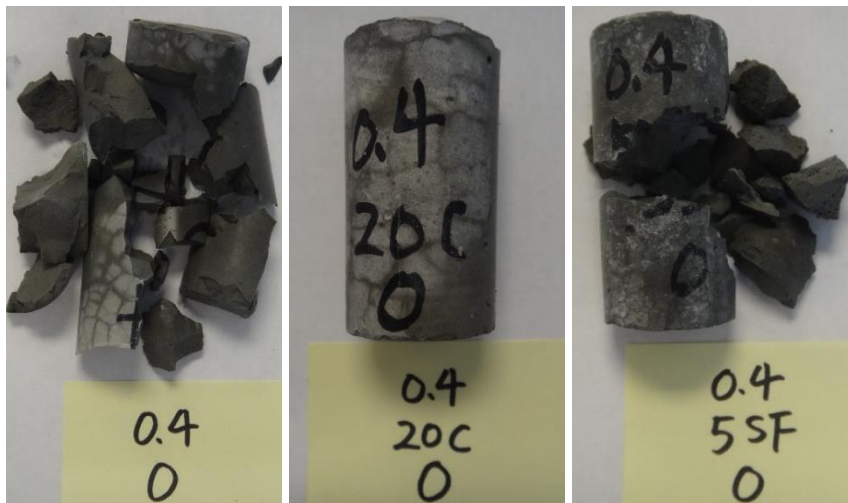
Figure 50. Oven dried paste samples with different SCMs after one freeze thaw cycle
