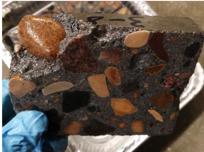
Figure 40. Sample exposed in 3% NaCl solution shown washed aggregate on concrete
