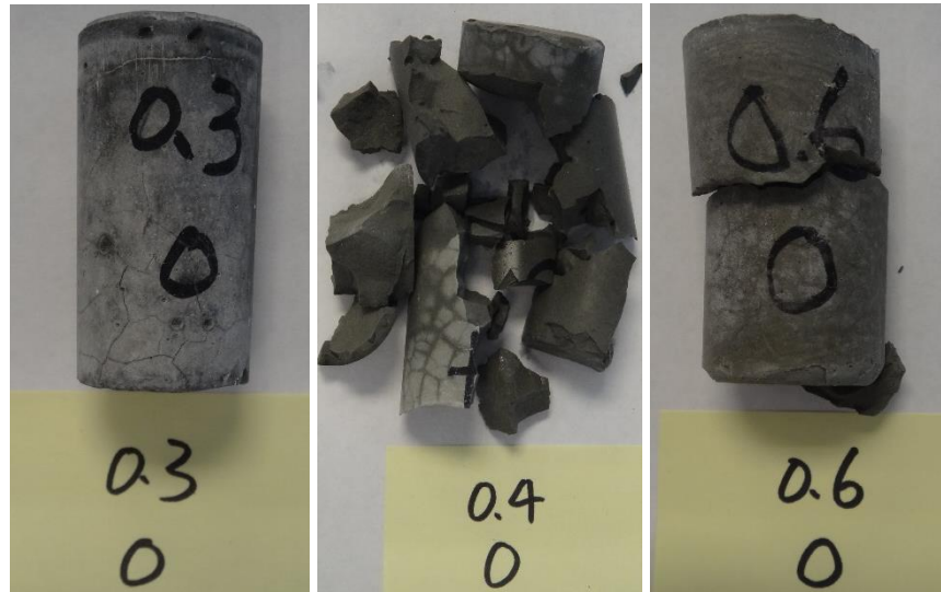
Figure 47. Oven dried paste samples with different w/cm ratios after one freeze thaw cycle
