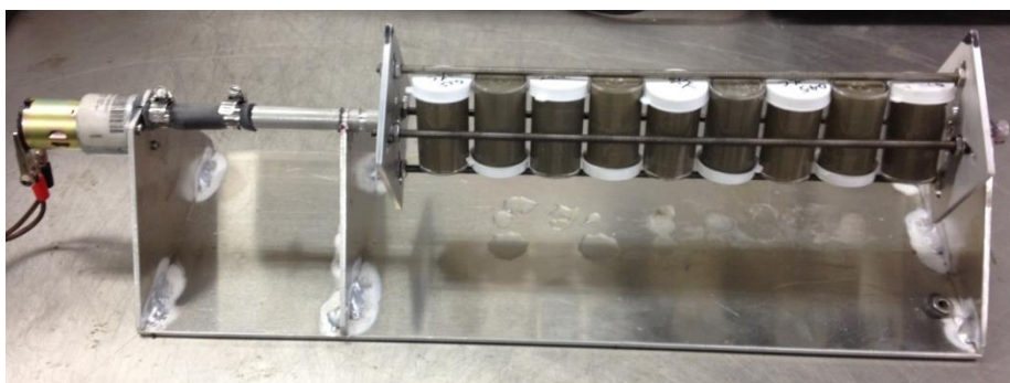
Figure 45. Rotating frame for fresh paste specimens during setting
