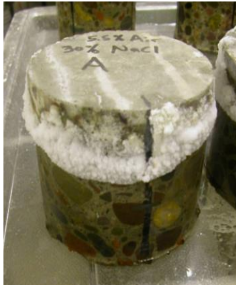
Figure 16. Typical example of concrete wicking
