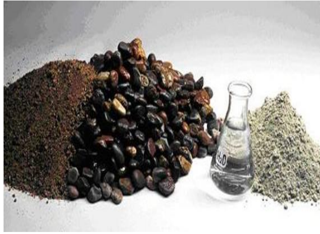
Figure 1. Composition of concrete
