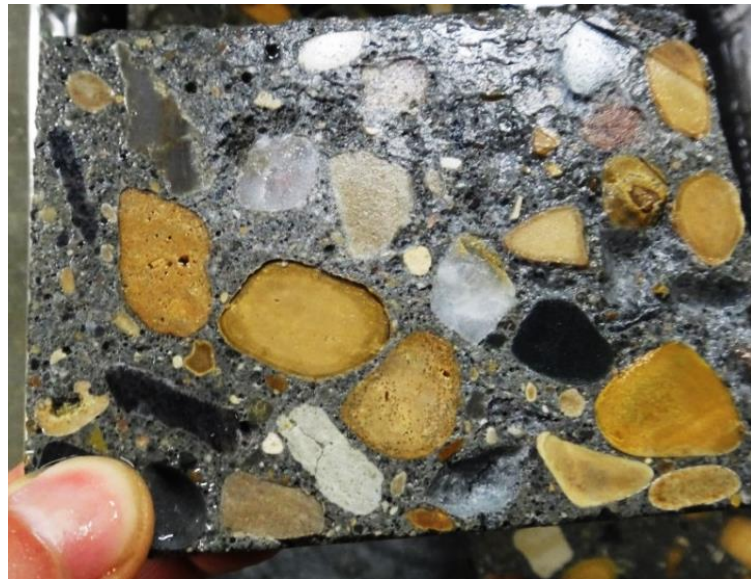
Figure 39. Sample exposed in water during freezing and thawing showing paste pushed above the aggregate
