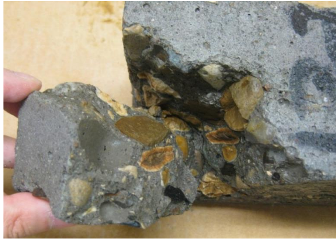
Figure 33. Laboratory observation of distress related to the ITZ during freezing and thawing cycle
