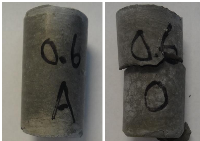
Figure 52. Comparison of freezing and thawing resistance for paste samples treated with different drying conditions
