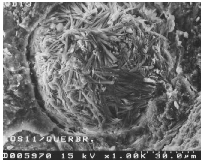
Figure 74. Air voids filled with ettringite in a damaged concrete pavement (Stark and Bollmann 2000)
